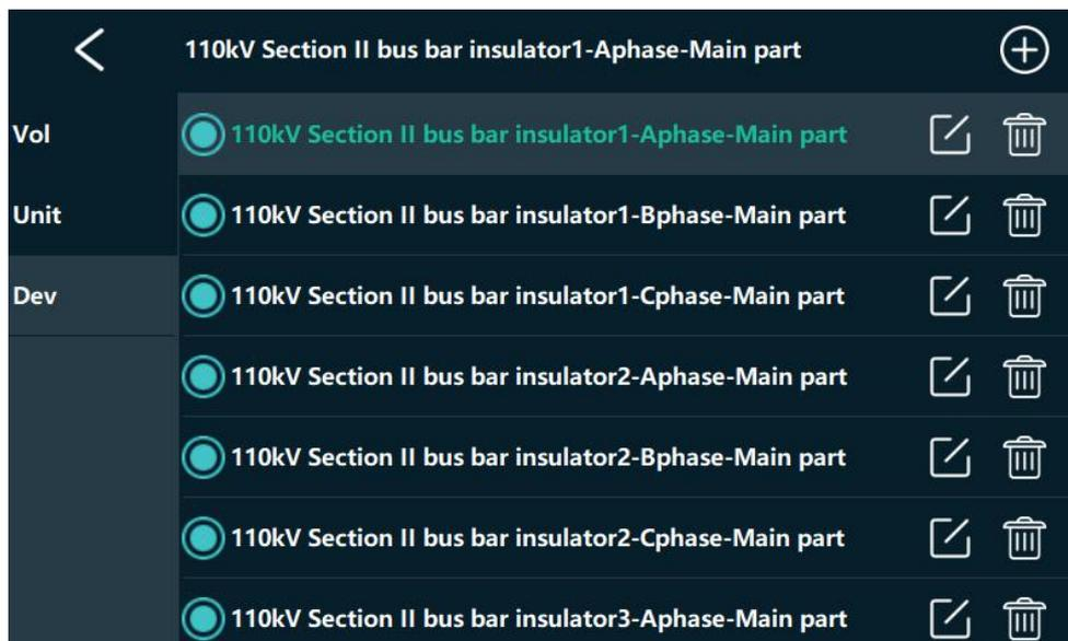
The system will name the images after the format of date + device name automatically when the image is saved.
