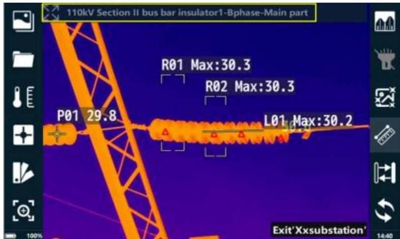
The image will be captured in order of smart image capture package in default. The user can click the device names as illustrated in the above yellow box and select the capture target in the pop-up device lists. See the below picture.
