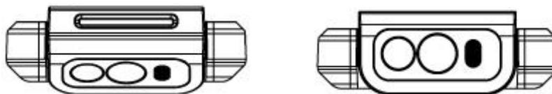
The lens module can be rotated at angles of 0°, 30°, 60° and 90°. Please do not rotate more than 90° to avoid damage to the camera.
