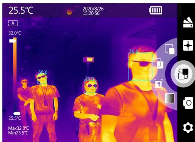
The screen displays temperature, power, date&time, temperature bar and the main menu below the main interface. The main menu includes five functions: photo viewing, image mode, temperature measurement tool, color palette, and setting. The fan-shaped menu displays the secondary menu in the central of the main menu.
