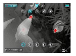
pressing the **Down (6) button** to change the image contrast level from 1 to 5 in the shortcut menu 2.
