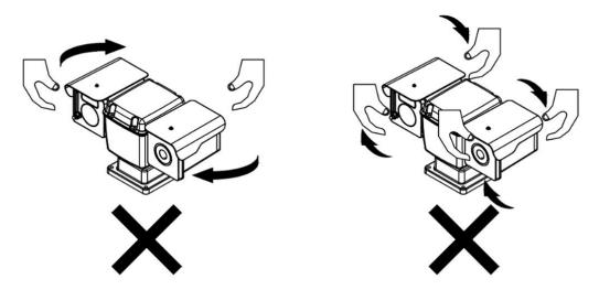
In order to avoid device damage, do not rotate the PT with big strength from vertical or horizontal direction during power-off state. The PT position can be changed via control interface.
