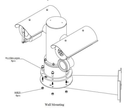
Figure 2.1 Fix the PT on the Base
