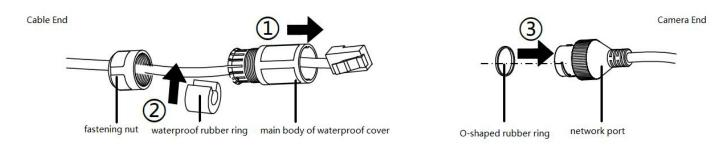
Figure 2.2 Network Cable Installation
