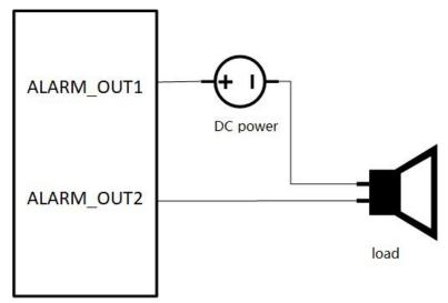
Figure 1.3 Alarm Output Wiring Method
